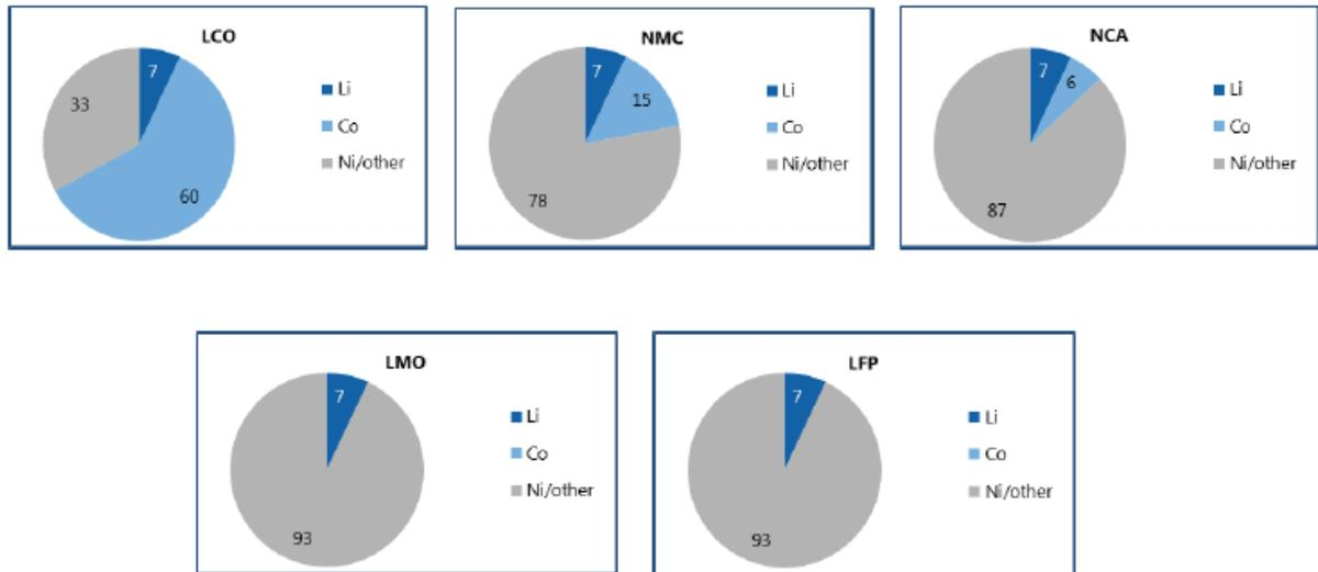
Figure 3: Material Content of Lithium-Ion Battery Types (%)<sup>19</sup>
