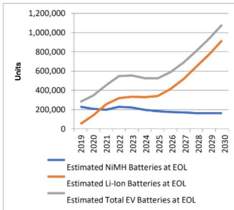
Figure 4: Estimated EV Batteries Reaching EOL in the US, by Battery Chemistry (2019-2030)
